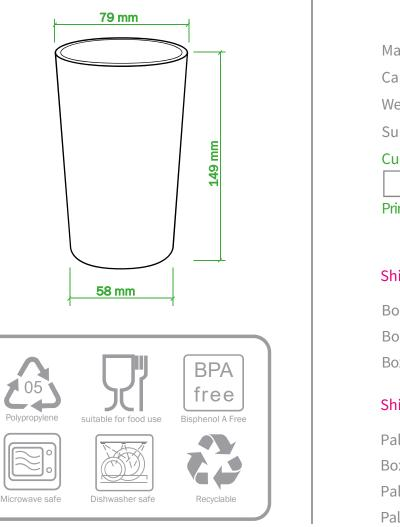
Material: Homo polypropylene Capacity: 50 cl Weight: 42 gr Surface finish: Translucent
